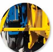
Extended debris shroud helps to keep refuse in the hopper.
